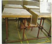
WPC boards are available with various names like 'Construction boards', 'Crust foam boards', 'Calcium boards', 'WPC shuttering boards' 'WPC MDF boards' in global markets. WPC boards can be produced with flexible density range varies from 400 kg/cum to 900 kg/cum. Another important characteristic is the surface density of this product and which also can be adjusted between a range of 55 shore D to 85 shore D surface hardness.
